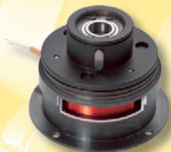
The basic model of electromagnetic clutch with bearing consists of stator body ① with cast-in coil and connection cable ②, the input drive hub ③ with support bearing, and the armature disc ④ to which the return spring ⑤ is riveted. Because it contains a bearing, it is not necessary to centre the stator body on the input drive hub when using this model.
