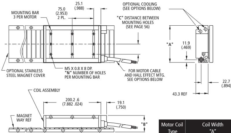
Resultant airgap = 0.9mm (.036) nominal (0.5mm (.020") minimum) when components are set up to dimension "B" in table below. (Please refer to installation manual for more detail)
