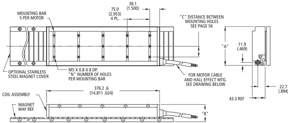
Resultant airgap = 0.9mm (.036) nominal (0.5mm (.020") minimum) when components are set up to dimension "B" in table below. (Please refer to installation manual for more detail)
