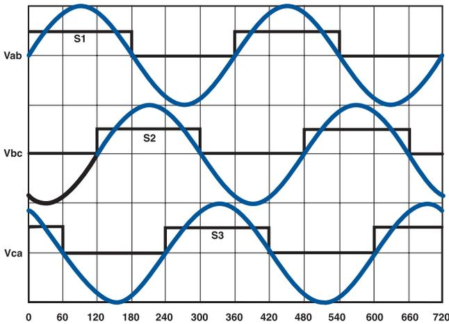
• Motor BEMF phases A,B,C relative to Hall effect devices S1,S2,S3 with coil travel direction towards the motor output cable assembly exit as shown below.
