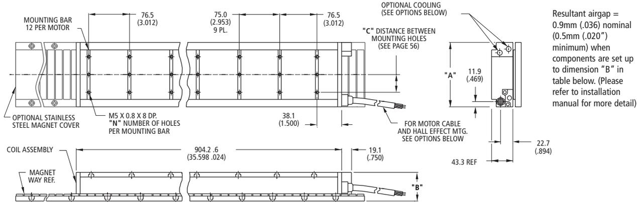
Resultant airgap = 0.9mm (.036) nominal (0.5mm (.020) minimum) when components are set up to dimension "B" in table below. (Please refer to installation manual for more detail)
