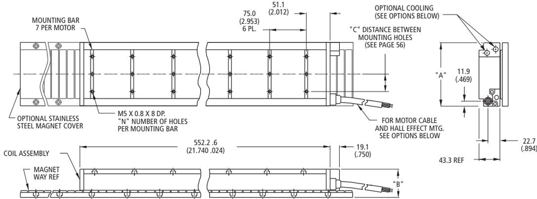
Resultant airgap = 0.9mm (.036) nominal (0.5mm (.020") minimum) when components are set up to dimension "B" in table below. (Please refer to installation manual for more detail)
