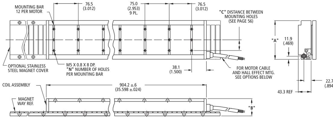
Resultant airgap = 0.9mm (.036) nominal (0.5mm (.020") minimum) when components are set up to dimension "B" in table below. (Please refer to installation manual for more detail)
