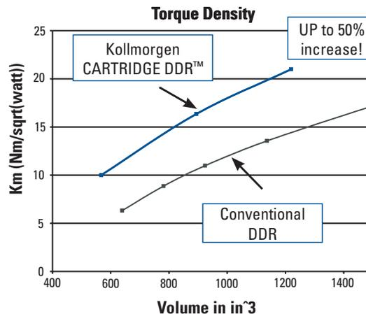
Proprietary electromagnetic design gives CARTRIDGE DDR™ motors more torque per volume than conventional DDR technology.
