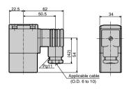
T terminal box (G1/2) T terminal box (७١/८, NVP11-10A/15A/20A/25A-1 3T 3R
