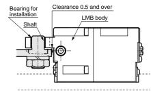
Insert a shaft (pin) into the bearing for installation and connect to the slide table. Provide the clearance shown above. Due to the structure, the LMB moves up and down during locking, so if bearings are fixed without clearance, the lock is not applied.
