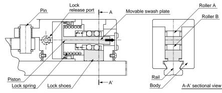
When the lock release port is pressurized with air, the piston and the tapered movable swash plate connected to the piston move in the direction of the arrow, releasing contact between roller B and the movable swash plate.
