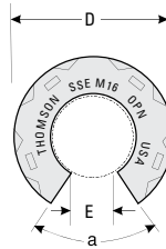
Super Smart Ball Bushing Bearings (Open Type) (Dimensions in mm)
